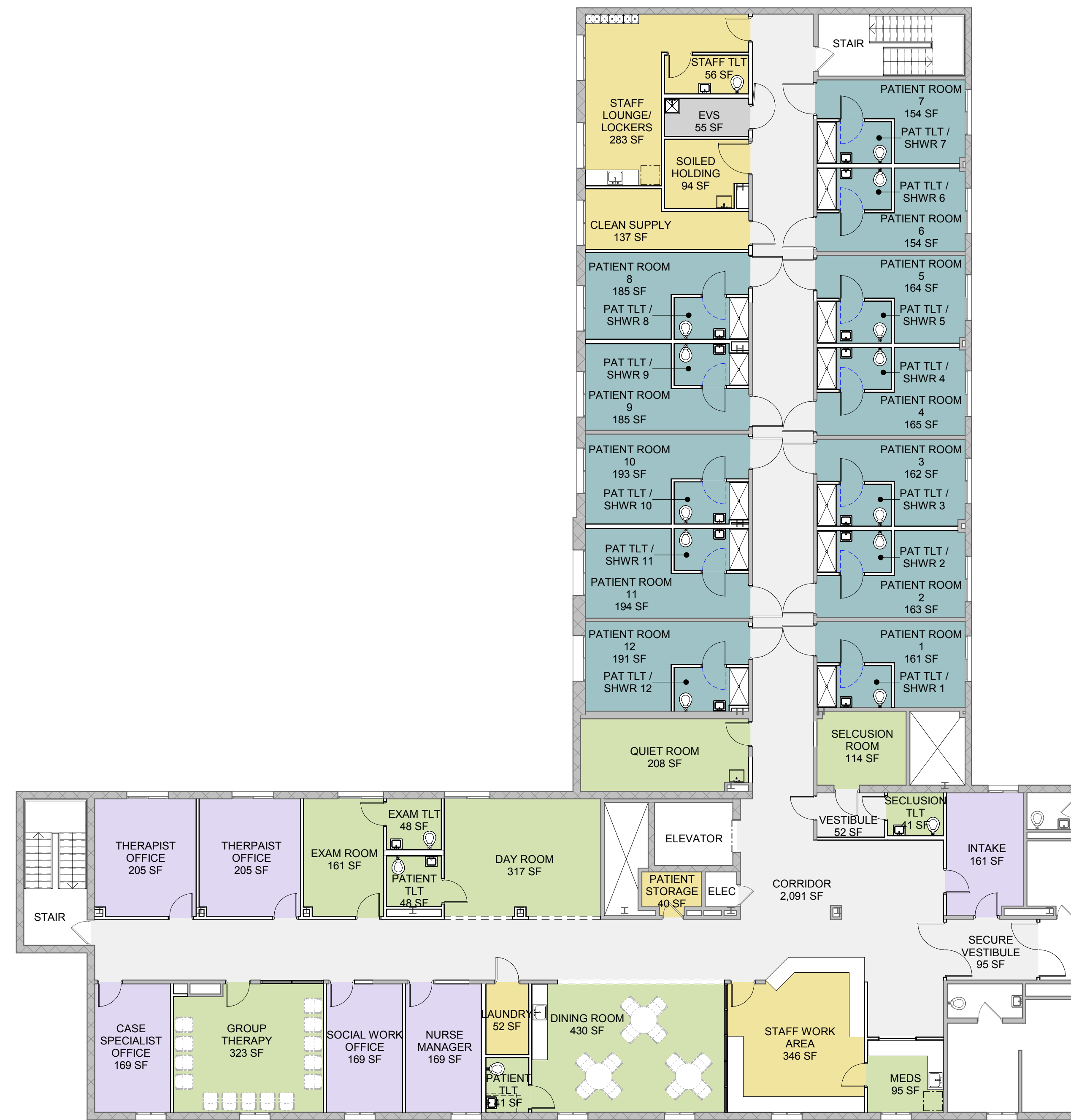
2 THIRD FLOOR - PROPOSED CONSTRUCTION SCALE: 3/32" = 1'-0"
