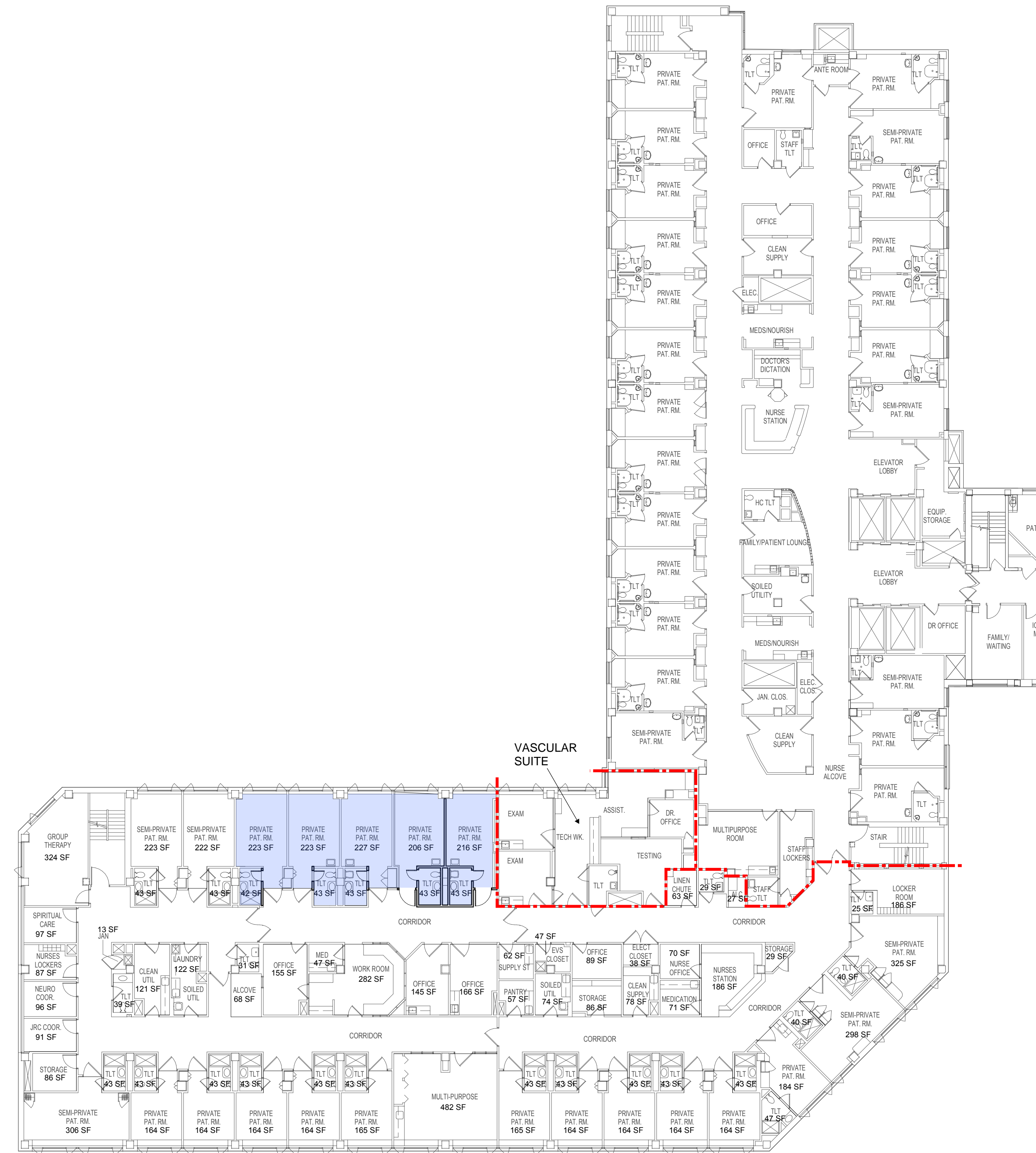
2 Level 04 - Proposed 1/16" = 1'-0" 5 NEW PRIVATE MED/SURG PATIENT ROOMS ON LEVEL 4 SOUTH LEVEL 4 EAST TO REMAIN AS EXISTING
